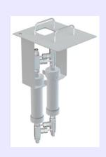
Combination of lids offers several possibilities for this D1838 setup. For example the combination enabling two or four positions for LPG test cylinders.
